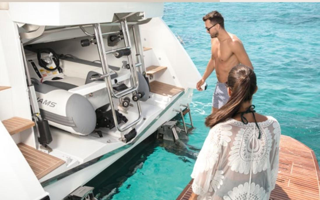
The tender garage at the stern, compatible with the Williams Minijet 280, holds any standard outboard tender up to 2.90 m and opens onto a huge submersible swim platform. Withstanding up to 350 kg, this platform is ideal for any water sport equipment. Launching is made easy with a hydraulic system that quickly raises and lowers your leisure equipment.
