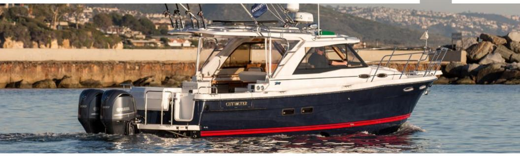
**The new Cutwater 302 Sport Coupe** (C-302 SC) is an exciting take on our successful Cutwater 30 family cruiser. The Cutwater 302 Sport Coupe is named for its open design that truly invites the outside in and keeps you close to the action. The C-302 SC is powered by twin counter-rotating Yamaha 300 HP outboards that push its double-stepped hull effortlessly across the water. The new C-302 SC hull also incorporates our patented Laminar Flow Interrupter technology for smooth, positive cornering.
